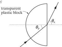
A student traces the path of a narrow beam of light through a transparent plastic block, and measures the angles  $\theta_a$  and  $\theta_p$  (see diagram). She repeats the measurements for various chosen values of  $\theta_p$ , and her results are plotted below.
